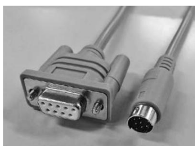
Figure 6.31: Serial port on the DTM sound source and the connecting serial cable
