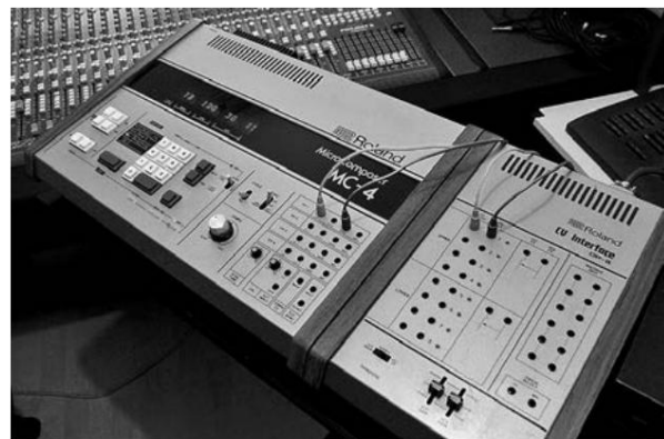
Figure 2.18 Example of connection between Roland OP-8 and OP-8 and MC-4
